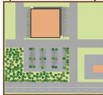
Utilize maximum number of parking spaces and require that landscaping be used as a buffer between the parking lot and the arterial.
