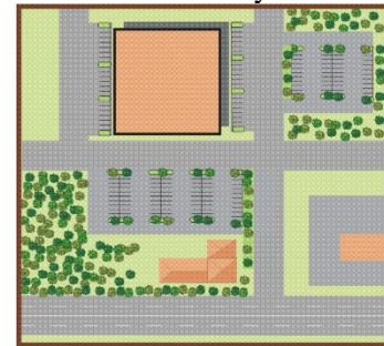
Compartmentalize the parking by breaking up into compartments with a maximum number of spaces.
