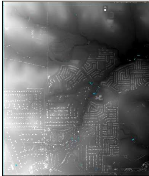
Figure 29 - Tile u329705_2_b; an example of first-return model showing NoData areas in bright blue
